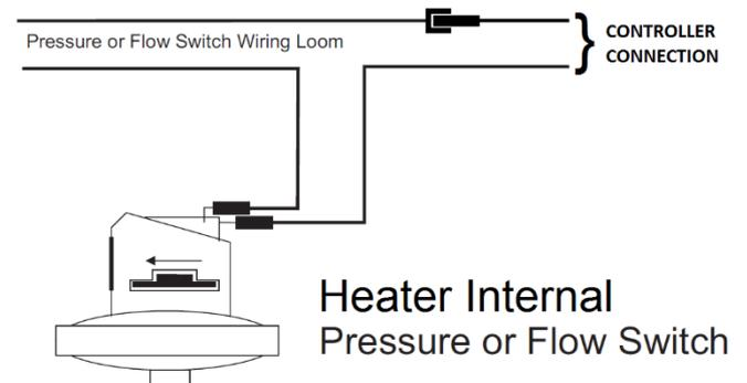
Internal connection to pool heater [check with heater manufacturer].
